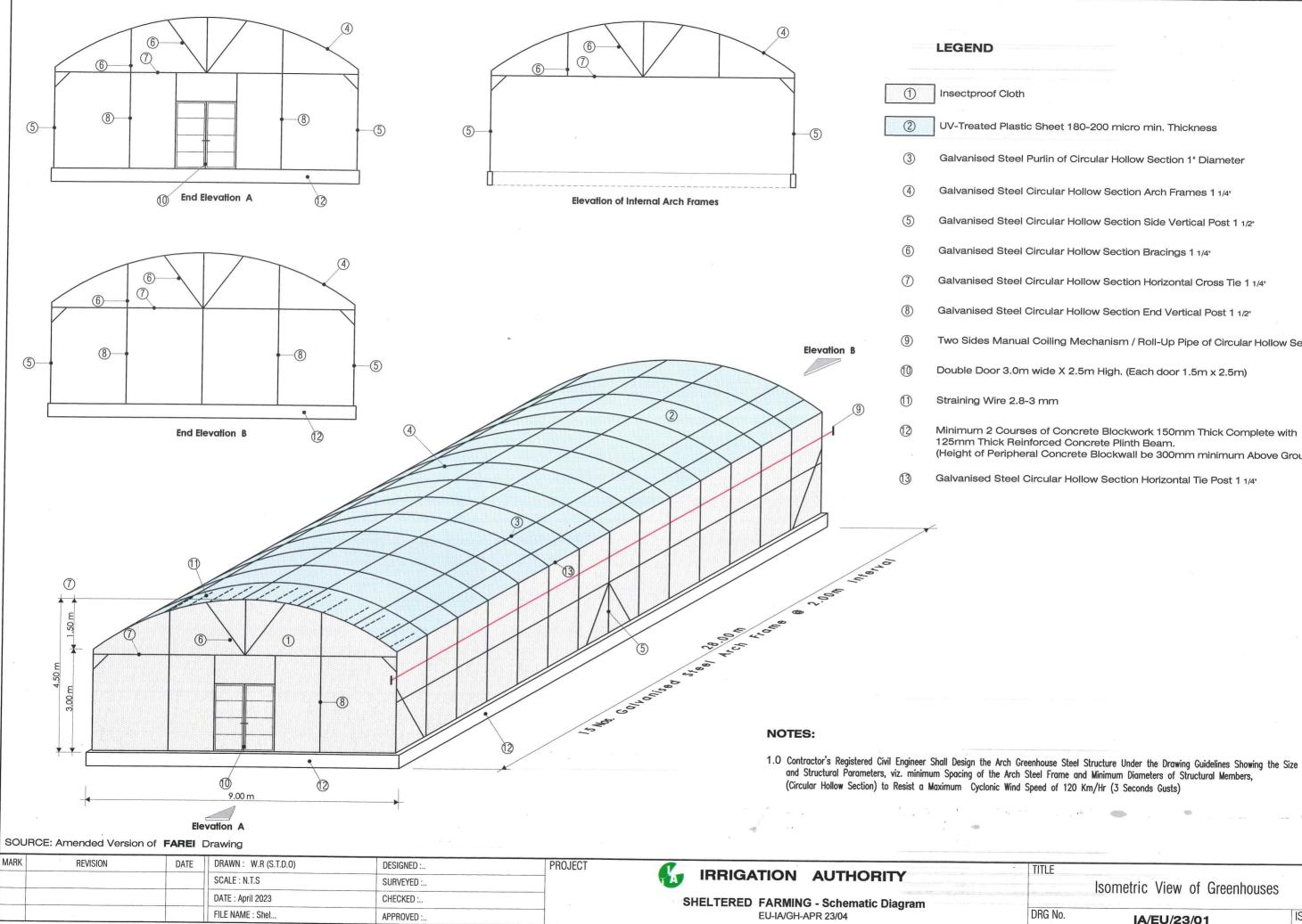
UV-Treated Plastic Sheet 180-200 micro min. Thickness
